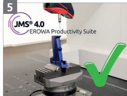
05 | The result „within tolerance“ or „incorrect workpiece“ is automatically stored in the process control system.
